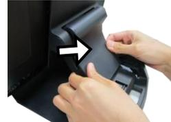
4. Tilt the terminal to the horizontal position. Then, thread cables through the cable passage.
